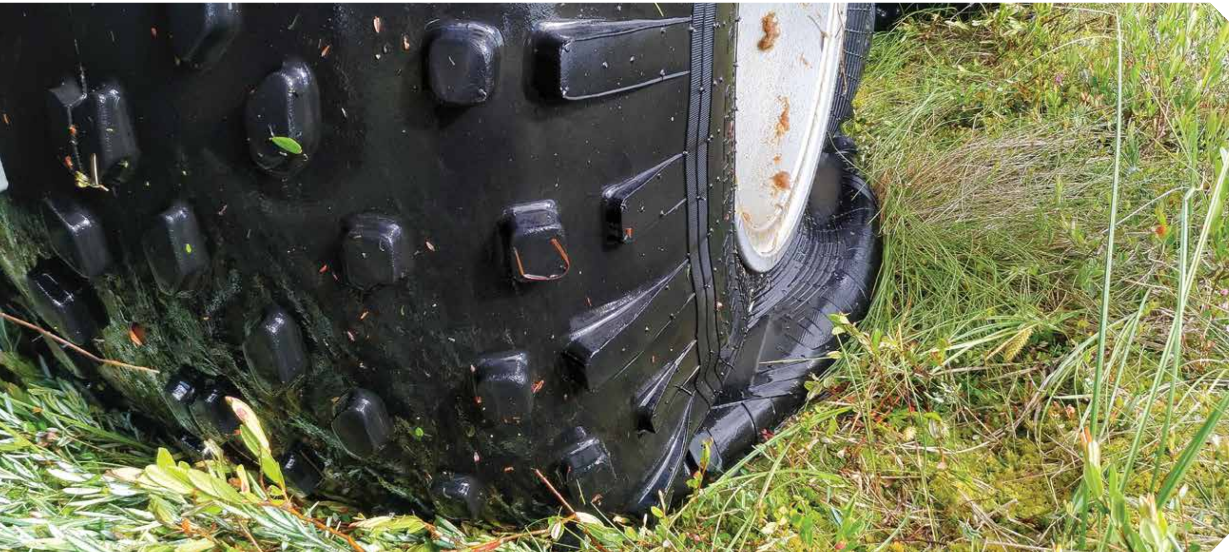
AVTOROS MAX-TRIM tire in the «Swamp» mode, pressure 0.05 atm
